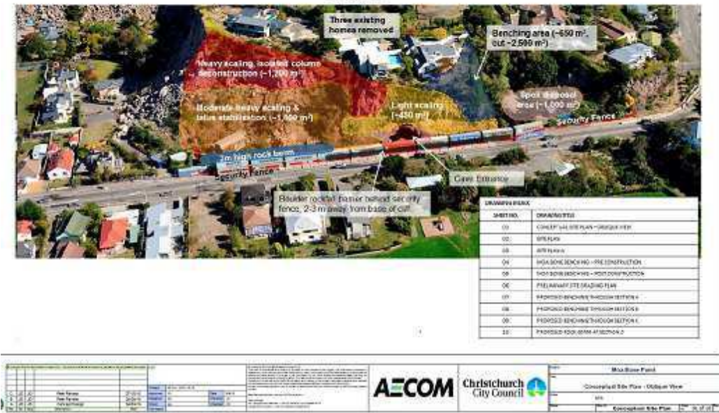
Overview of planned works at Moa Bone Point. Note the line of containers which had to be removed for work to start. A planning note Moa Cave says “Debris at cave entrance to be re-shaped.”
